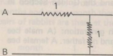
$n$  units like this are joined to form a ladder network. If each resistance is 1 ohm, what is the total resistance  $r_n$  between A and B?
